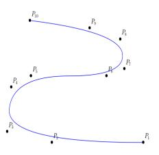
The curve after duplicating the multiplicity of the internal knots  $\{\frac{1}{4}, \frac{1}{2}, \frac{3}{4}\}$ , this leads to a B'ezier description. We can then, split the curve into 4 pieces (sub-domains), each one will corresponds to a quadratic B'ezier curve.
