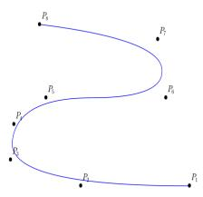
The curve after a p-refinement, the degree was raised by 1 (using cubic B-splines).
