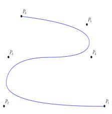
The curve after a h-refinement by inserting the knots  $\{0.15, 0.35\}$  while the degree is kept equal to 2.
